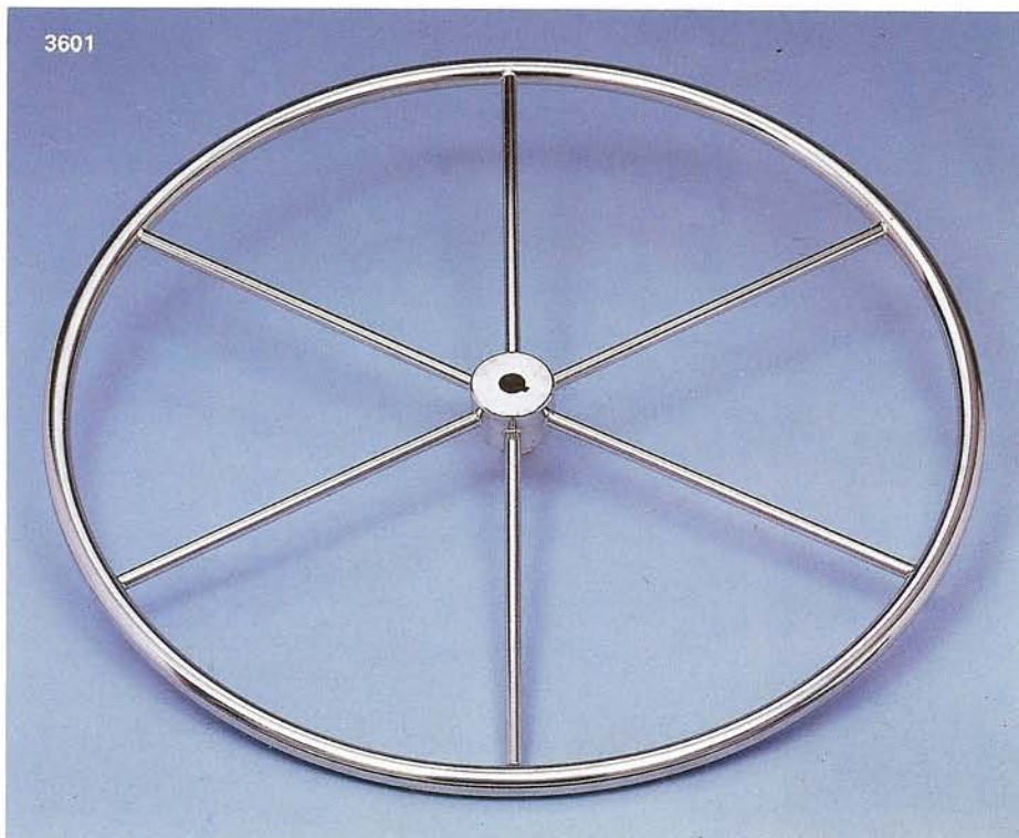
3601 STEERING WHEEL 駕駛盤 Material: SS Hub Length: 2 1/8" (54mm) Key: 1/4" x 1/4" (7mm x 7mm) Available Size: 26", 28", 30", 36"
