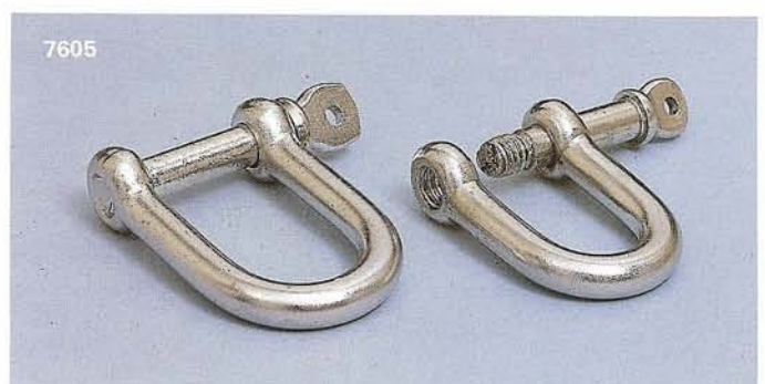
7605 FORGED "D" SHACKLE 縮果" Material: SS SIZE: 3/4" x 1 7/16" x 5/16" (19mm x 37mm x 8mm) 1" x 1 1/2" x 5/16" (25mm x 38mm x 8mm) SWL/Breaking Coad 7260 "lb"
