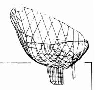
Her performance to weather is clearly superior to most vessels of this type due to my treatment of the keel. With her generous rudder and cutaway forefoot, she maneuvers easily yet the lateral plane of the keel is still sufficient to ensure self-steering qualities.
