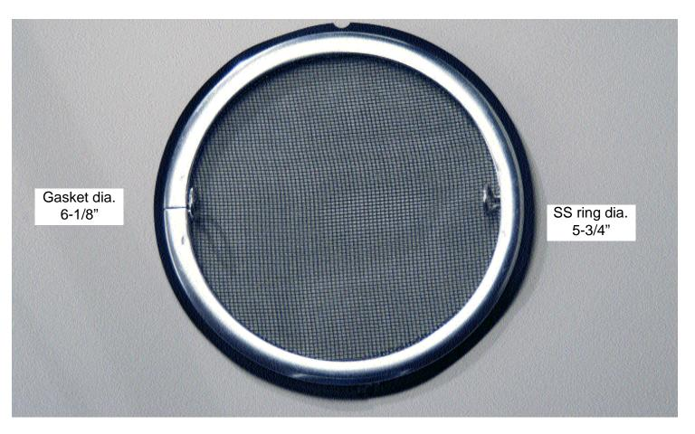
Screens are made up of two rings of stainless steel with a rubber gasket and a layer of nylon mesh screen sandwiched between. Screen material is not extremely fine mesh. Handles on sides allow for easy removal. They fit my T-37 extremely well.
